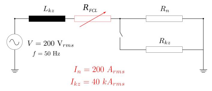
With fault current limiter In  $L_{kz}\frac{di}{dt} = V - [R_{kz} + R_{FCL}(T)]i$ ter
